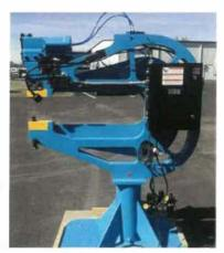
We were able to shave off over 1000lbs from this pneumatic press with our Waterjet so it could be installed on the third floor of a manufacturing facility. We solve unique problems on a regular basis at Industriol Resources, Inc.
